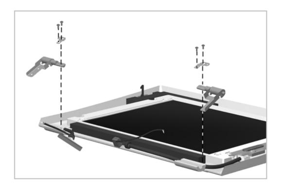
Figure 5-34. Removing the Clutch Assembly and Bracket Reverse the above procedure to install a clutch assembly and bracket.
